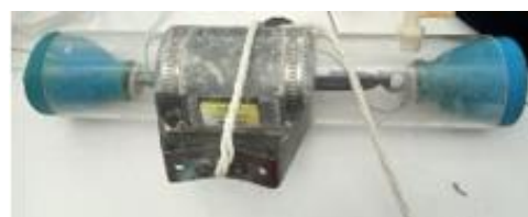
Figure 2. Van Dorn Sampler: (a) Schematic of the device; (b) Documentation of the device
