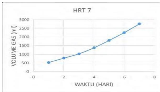
Figure 3. Effect of Hydraulic Retention Time (HRT) of 7 Days on Accumulated Biogas Volume
