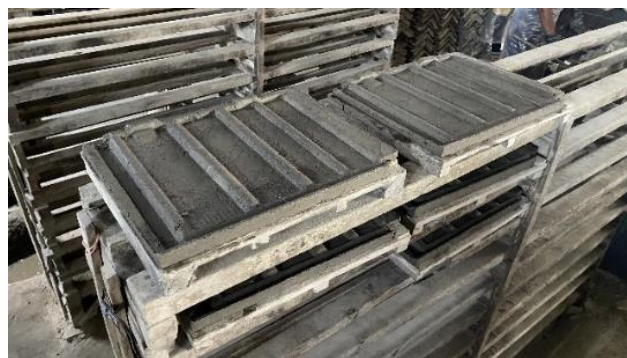
Figure 2. Concrete tile made from a mixture of medical waste incineration residue
