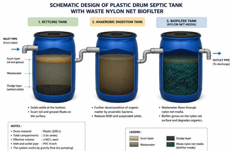
Figure 1. Schematic Design of Plastic Drum Septic Tank with Waste Nylon Net Biofilter
